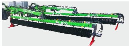
For superior control, the brush is equipped with a proportional valve, allowing precise adjustments for smooth and efficient operation. Additionally, a joystick control ensures effortless maneuverability.
